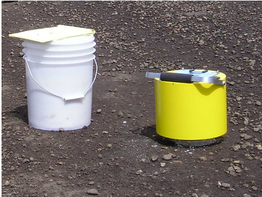
FIGURE 2.4 Soil stiffness gauge.
