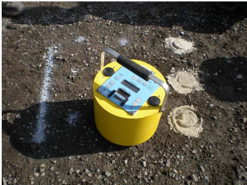
FIGURE 3.3 Testing with SSG to assess operator effects.
