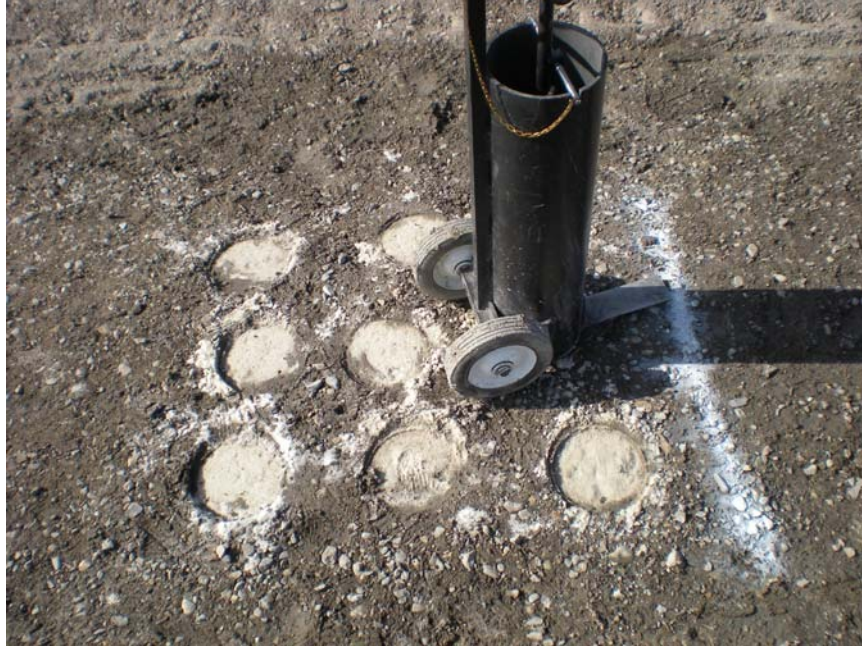
FIGURE 3.4 Testing with CIST to assess operator effects.
