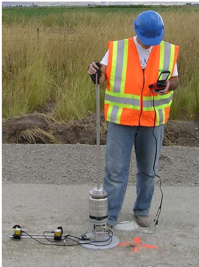
FIGURE 2.5 Portable falling-weight deflectometer.
